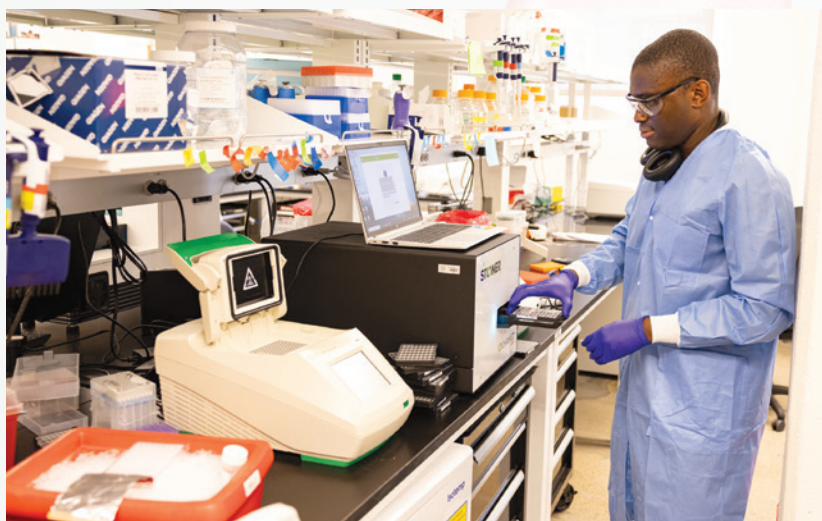
Christopher Duncan–Lewis, a scientist at Scribe Therapeutics, loads a microplate into a machine used to quantify the concentration of RNA extracted from cells.
