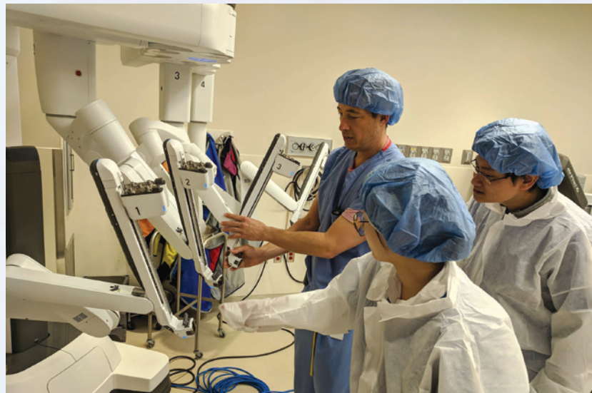
Ronald Boris explains the dynamics of the robotic patient cart, which holds the camera and instruments that the surgeon controls from the robotic console used for kidney tumor removal, to Purdue graduate students Peipei Zhu and Marco Hadisurya in the surgical room.
