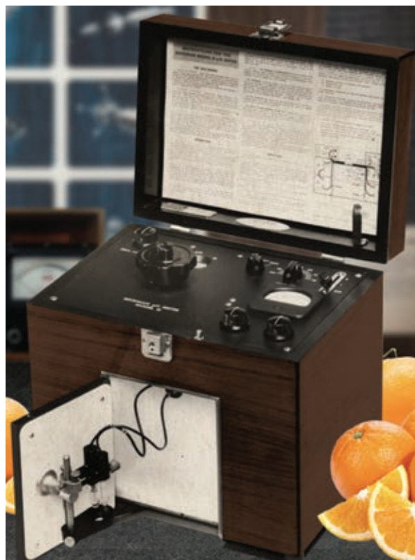
Arnold Beckman invented this model G pH meter in the 1930s at the request of a chemist from the California citrus industry who needed an accurate way to measure the acidity of his product.
