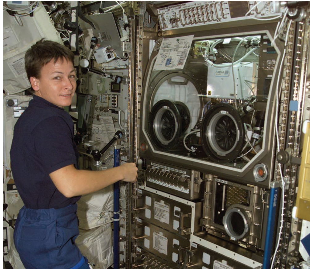
Astronaut Peggy A. Whitson works near the Microgravity Science Glovebox in the Destiny laboratory on the International Space Station.
