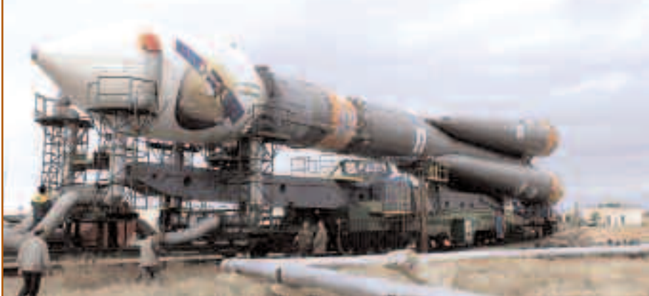
The Soyuz launcher during transport to the launch pad. Credits: ESA/STARSEM-S. Corvaja.
