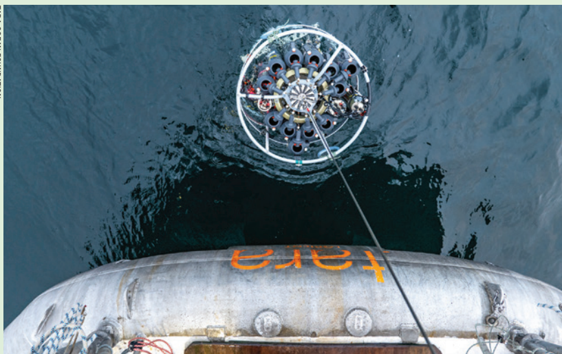
The Tara collects water samples from 1,000 feet below the surface using Niskin bottles in a carousel that resists water pressure and collect samples at specific depths without them mixing with water from other depths.
