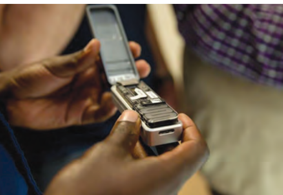
Commercially available nanopore DNA sequencing devices, such as this MinION device from Oxford Nanopore, are small and highly portable.
